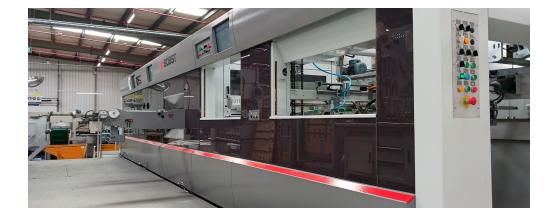
We replaced the two old machines with one flatbed die-cutter. Not just any one, but really the Rolls Royce among die-cutters. The machine can output as many as 7.500 sheets per hour. Moreover, it can process sheets with a maximum size of  $1450 \times 1050$  mm.
